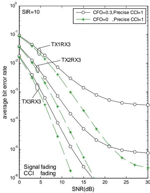
Fig. 2 Average BER for MRT-MIMO OFDM with CFO = 0 and 0.3. (SIR = 10dB)
