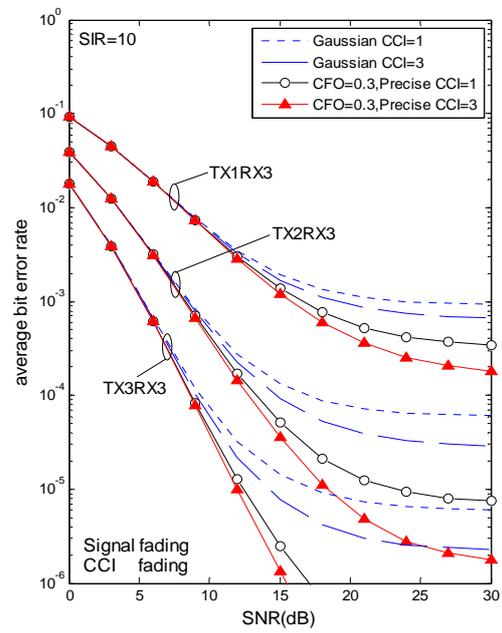
Fig. 3 Average BER for MRT-MIMO OFDM using precise CCI and Gaussian CCI models. (SIR = 10dB)
