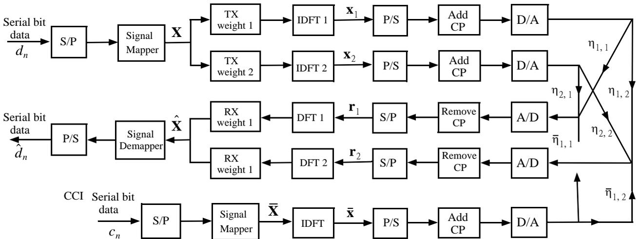
Fig. 1 MRT-MIMO OFDM (two transmit antennas and two receive antenna, one CCI)
