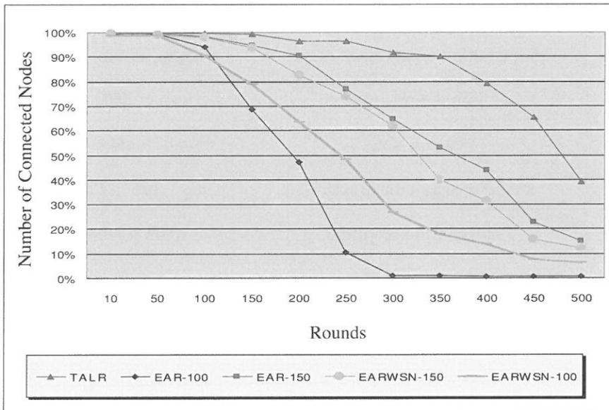
**Figure 5. System lifetime with 300 nodes**
