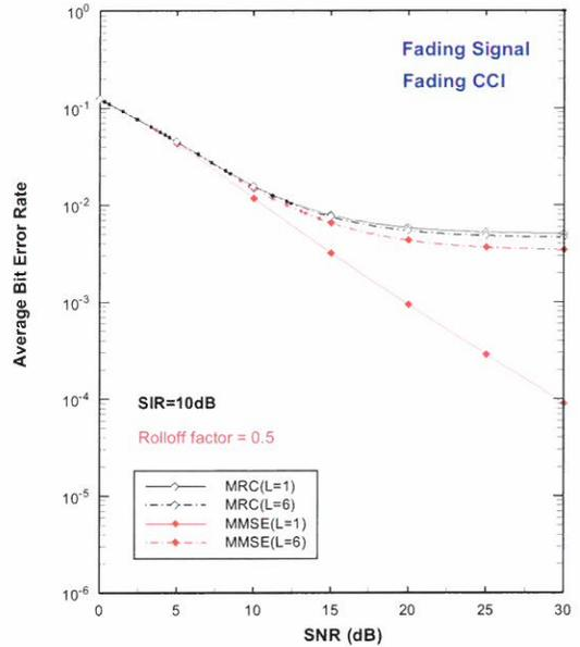
Fig. 6 Average error probability versus SNR for 4-QAM with MMSE combining and MRC combining at SIR=10dB (fading signal, fading CCI).
