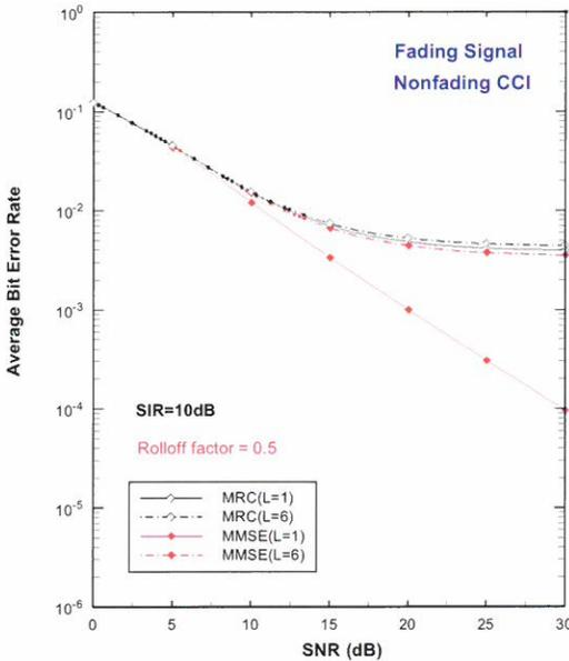
Fig. 5 Average error probability versus SNR for 4-QAM with MMSE combining and MRC combining at SIR=10dB (fading signal, nonfading CCI).
