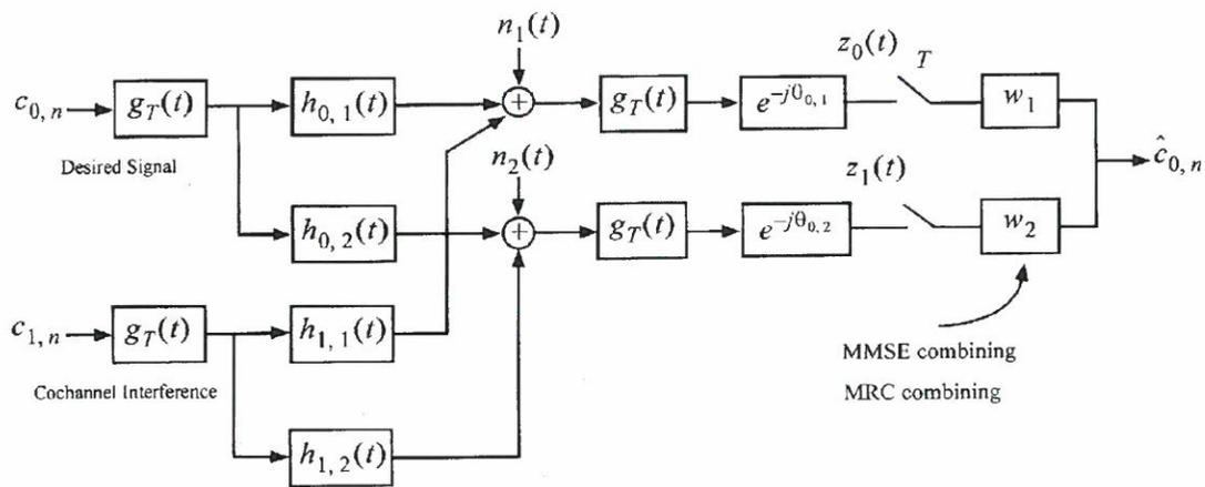
Fig. 1 Block diagram of the diversity receiver over a channel with CCI.
