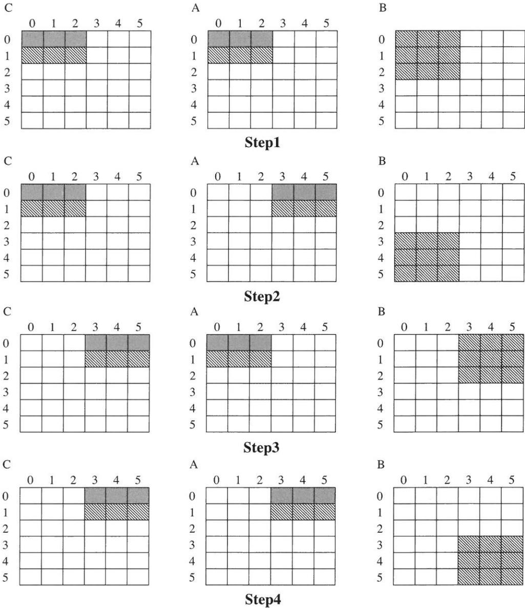
**Figure 4. The Process of Multithreading with Blocking Matrix Multiplication**
