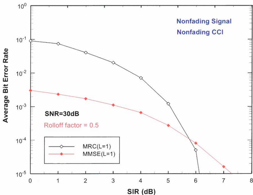
Fig. 2 Average error probability versus SIR for 4-QAM with MMSE combining and MRC combining at SNR=30dB (nonfading signal, nonfading CCI).
