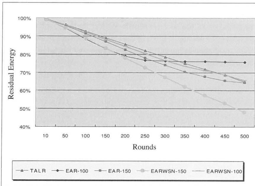
Figure 7. Residual energy by 300 nodes
