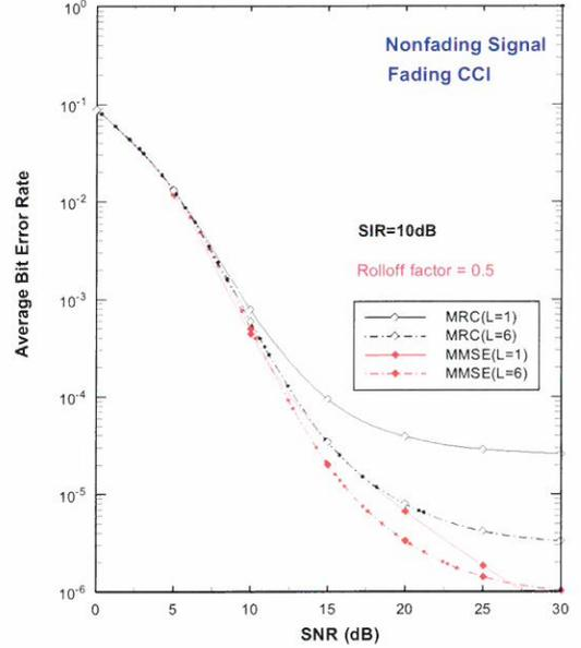
Fig. 4 Average error probability versus SNR for 4-QAM with MMSE combining and MRC combining at SIR=10dB (nonfading signal, fading CCI).
