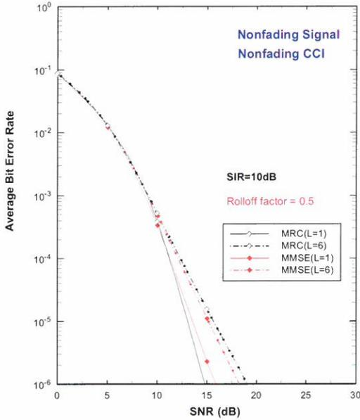
Fig. 3 Average error probability versus SNR for 4-QAM with MMSE combining and MRC combining at SIR=10dB (nonfading signal, nonfading CCI).
