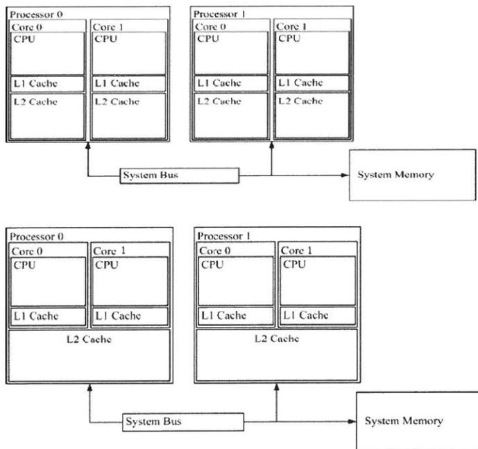
**Figure 1. Dual Socket System with Different Dual-Core CPU L2 Cache Organization (figure taken from [9])**
