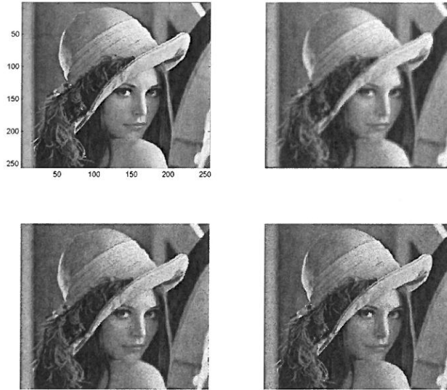
Figure 2. The top-left profile is the origin with noise. The top-right is for p=3 . The bottom profiles are p=4 (left) and p=10 (right). These results show the case of variance constraint.
