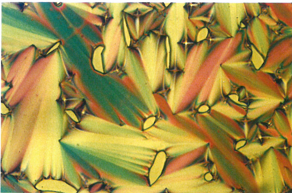
Figure 1. Focal conic fan texture of the mesophase of CnPNP, n=7 arises from isotropic phase on cooling to 82°C. Polarized optical micrographs with magnification of \times 400 .
