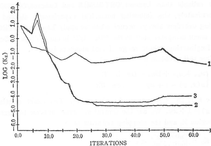
Fig. 1. Solving (2.1) with D = 5 and h = 1/8 by single precision. 1: Lanczos/ORTHODIR, 2: Lanczos/ORTHOMIN, and 3: Lanczos/ORTHORES.
